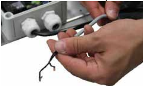
Figure 19: Disconnect the electrical wires from the water sensor connection and remove the cable.
