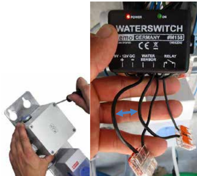
Figure 29: Changing the polarity of the electrodes.
