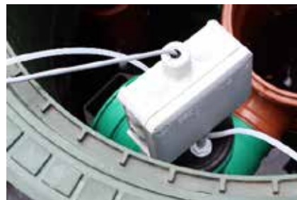
Figure 28: Position of the electrodes after installing the sensor unit back into the inflow pipe.
