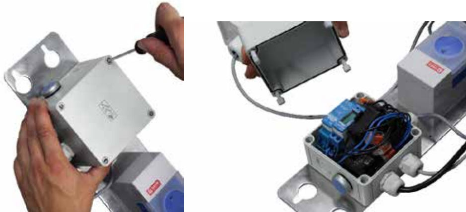
Figure 17: Opening the auxiliary control of the dosing unit.
