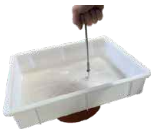
Figure 8: Mount the drip pan onto the plug connection in order to store the bleach solution inside the chlorine tank.
