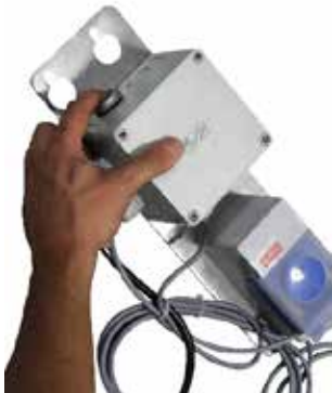
Figure 23: Integrated push button to fill the dosing hose with chlorine solution.
