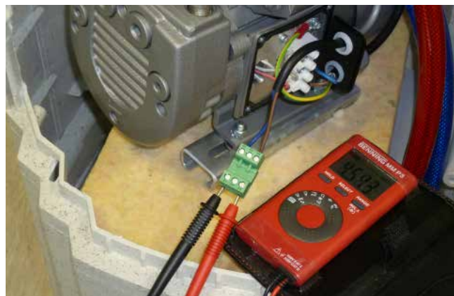
Measurement of the capacitor capacity for the rotary-slide compressor
