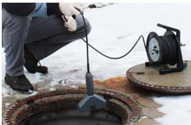
Measurement with the sludge-level measurement device
