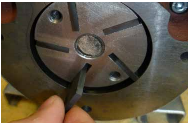
Checking the slider on the rotary-slide compressor
