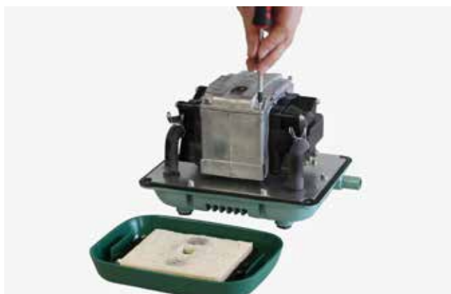
Remove the top casing part, sound-damper mat and inner casing cover one after the other.
