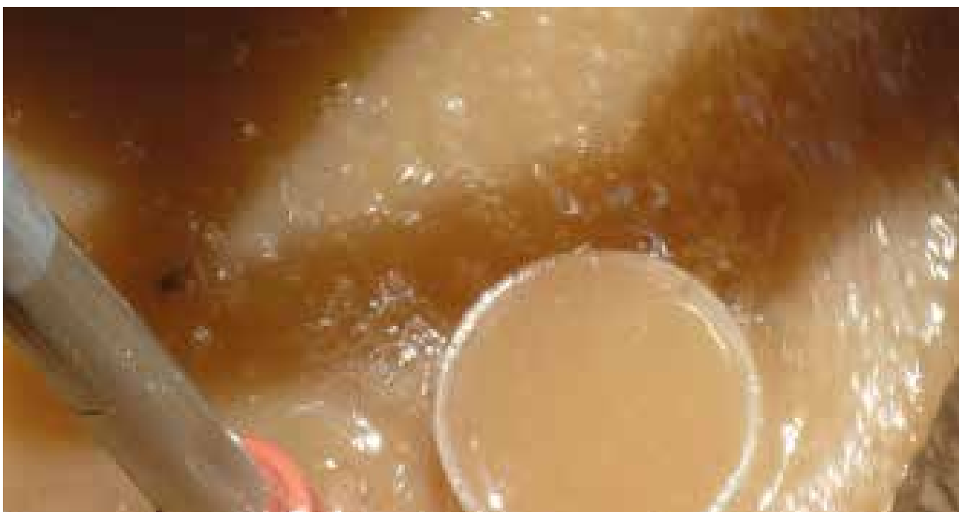
Extraction of a sludge sample from the activation basin
