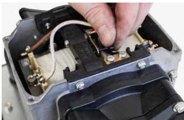
Insert the new safety pin. Just as for HP compressors, newer models have a safety switch rather than a pin.
