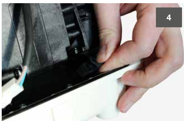
Remove the pump block from the lower casing part. Carefully remove the rubber buffers.
