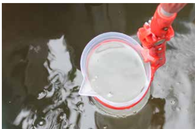
Outflow sampling after sufficient settling time
