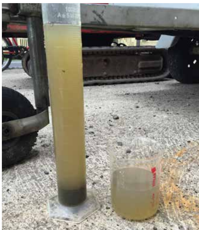
Poor water quality, strong opacity, little activated sludge, but lots of oxygen: inhibition likely
