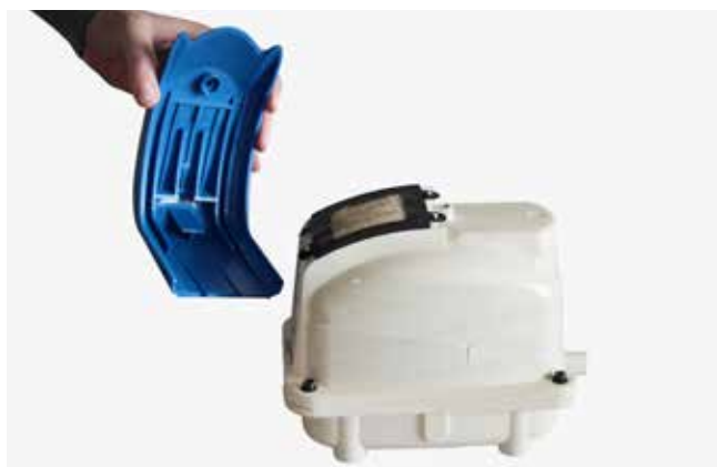
Removing and cleaning the filter cover
