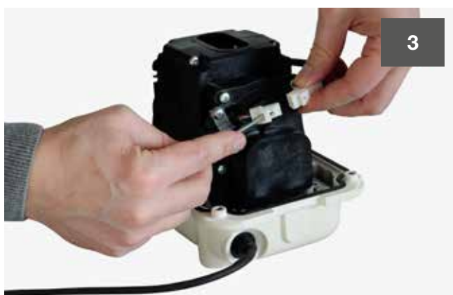
Remove the sound-damper mat. Release the plug from the fastening and decouple it.
