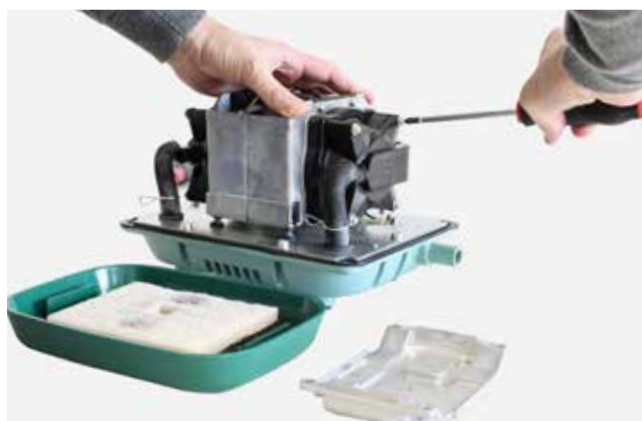
Loosen the L-shaped pressure connections. Unscrew and remove the pressure chambers on both sides
