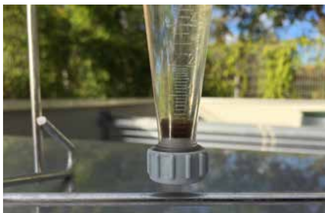
Measurement result after 2 hours of settling time in ml/l
