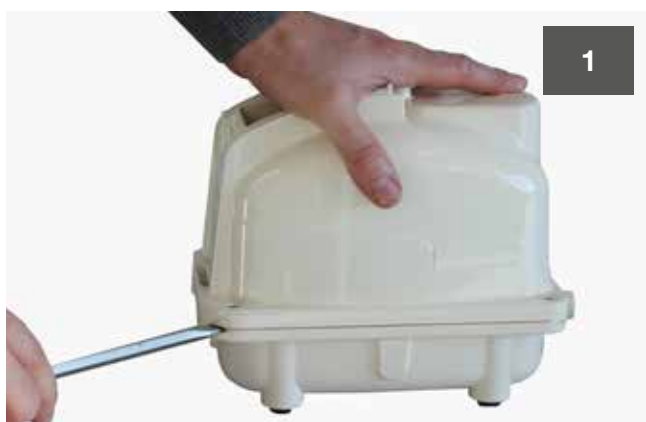
Unscrew the top casing part and remove. Pry it open with a screwdriver in case it is firmly attached.
