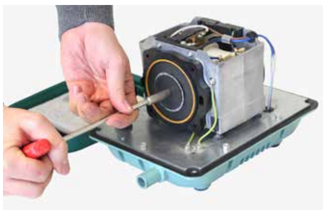
Unscrew and remove the membrane from the axle on one side
