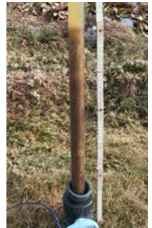
Sludge thickness is subsequently measured with a folding ruler.
