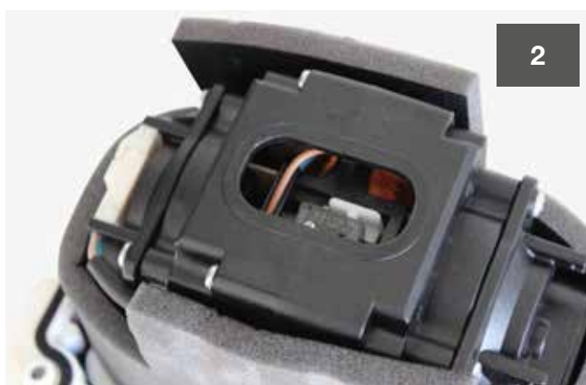
Remove the rubber cover. The safety switch is visible underneath. The white switch is off-centre, and the contact is interrupted in case of membrane breakage.
