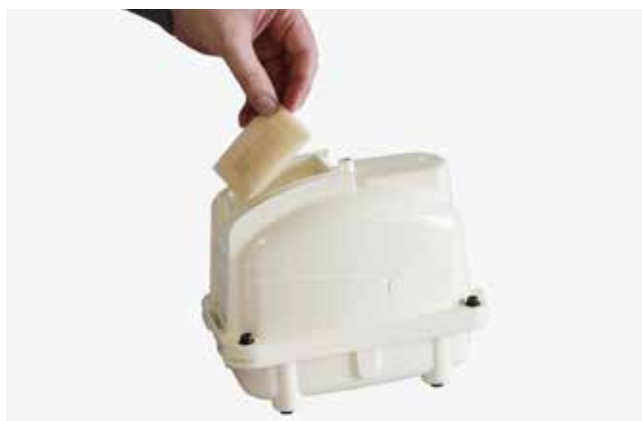
Removing gasket and filter, cleaning or exchanging the filter
