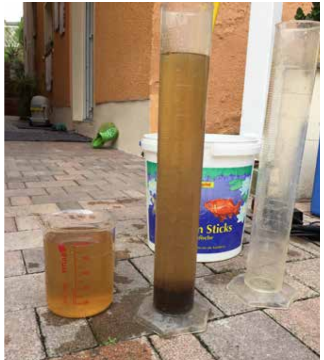
Strong opacity after settlement, only some of the activated sludge settles while the rest remains suspended.
