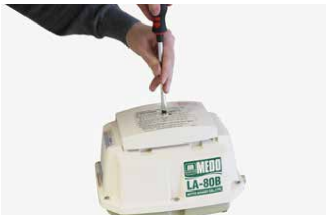
Unscrewing the cover for NITTO compressors
