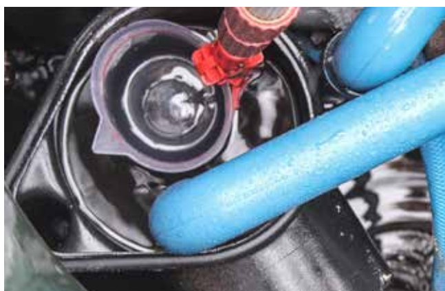
Outflow sampling without contacting the walls
