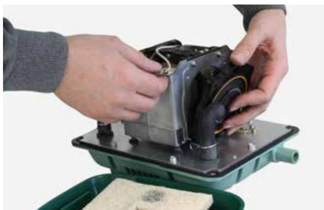
Exchange both membranes and seal rings. Assemble everything again.
