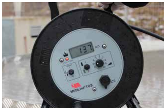
Thickness of the clear phase is indicated, sludge phase below.
