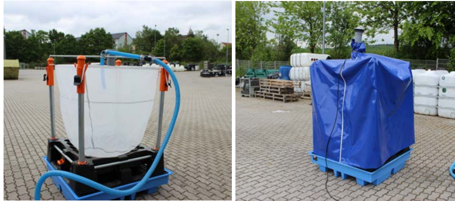
Figure 6: The filter unit consisting of collection tank, bag mounting, bag filters and cross member (left); filter unit covered with ventilation for drying (right)
