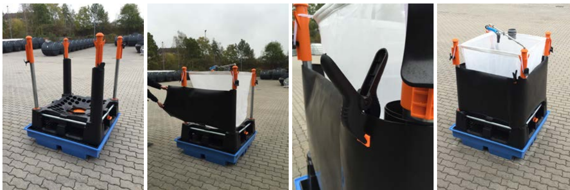
Figure 8: Attaching the splash guard (left to right): Winding the splash guard foil sheets on two opposite posts; pulling the sheets out; fixing with spring clamps; fully assembled splash guard
