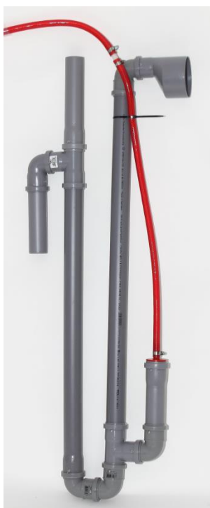
Lifter to feed the SBR reactor
