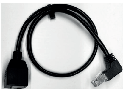
Illustration 3901475 Ethernet extension cable FTP Cat6 right-angled 0.5m (as standard for I-cabinet PP)
